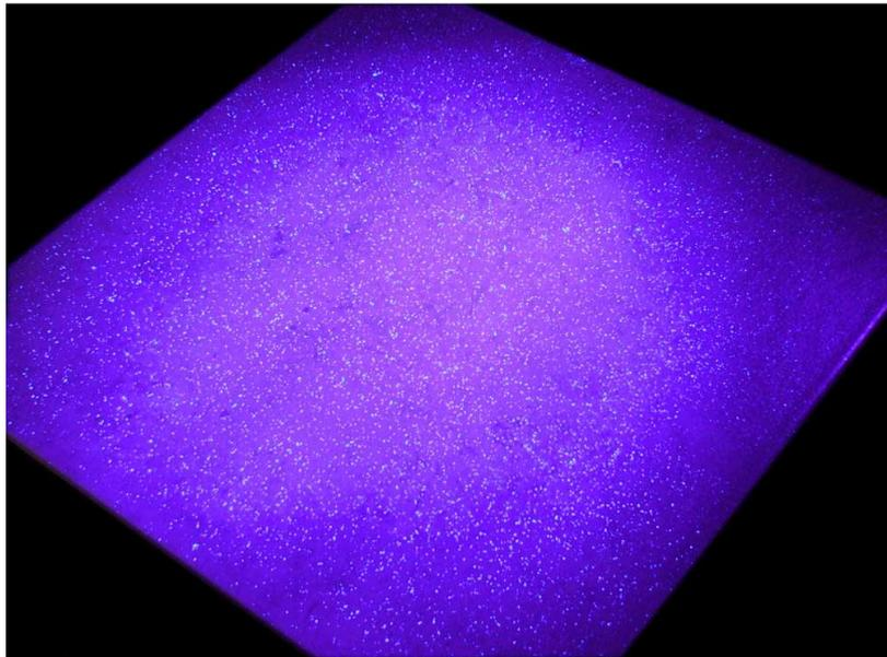
On certain surfaces, the Bactiscan is also capable of illuminating selective components of the surface matrix, for example Titanium Dioxide whitening agents in plastic and paints. Hard water scale also shows up as a blue – green colouration. Also optical brighteners used in papers and fabrics appear to fluoresce but at a different wavelength to micro-organisms.
